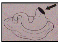
Bad impression: Canal too Short (Foam Stop not inserted deeply enough)
