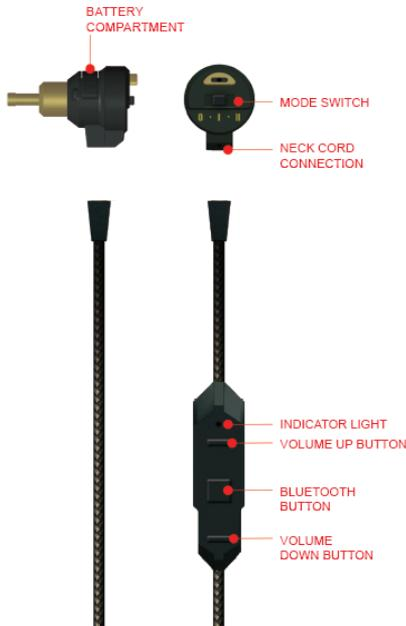
**NOTE: THE STEALTH ELITE HAS A BUILT-IN "SAFETY" CIRCUIT WHICH LIMITS THE OUTPUT OF THE INSTRUMENT TO A MAXIMUM OF 110dB SPL**
